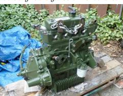
better and just needed to be touched up, while out I replace the gear-change bushes and added a magnetic oil trap. The front sub-frame was next, this was unassembled, each piece touched up, repainted, then reassembled and installed. Front brakes were next, the calipers were disassembled, painted, the seals were replaced and stainless steel pistons
