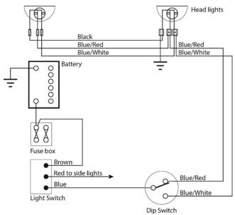
In the original circuit the power to the lamps, comes from the battery via the brown wire from the non-fused side of the fuse box to the lighting switch, on to the dip switch, where is splits into main and high beams.
