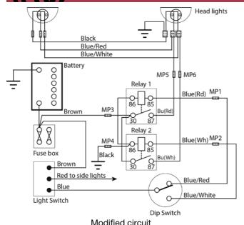
(MP1) - Disconnect the blue/red bullet connection to the lights, un-solder the bullet from the loom and replace with a female spade connector from the multi-plug (side A). This will determine the location of the multi-plug. Wire a male spade connector for the multi-plug (side B) to a 10A wire and run to coil terminal 85 of relay 1. Keep the bullet connectors safe as we will be re-using them later.
