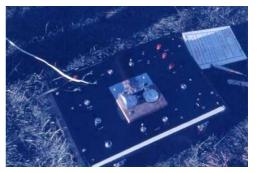
Timing gear – a pair of ordinary stop watches operated by the solenoids from a pair of trafficators, Telephone functions were incorporated for use at hill climbs but not being used at Levin.
