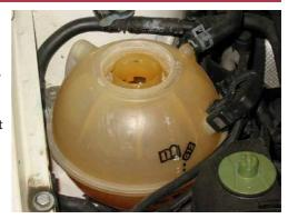
VW Polo double skinned coolant expansion tank
