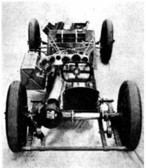
The chassis laid bare. Note the angle of the engine and transmission and the oblong steering wheel.
