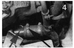
**Step 8.** Disconnect hose connection at the water pump (Photo 4).
