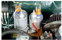
over, fingers crossed no leaks so far. The leak came from a pinhole where the cylinder body meets the reservoir. Impossible to detect until the system is filled and used.
